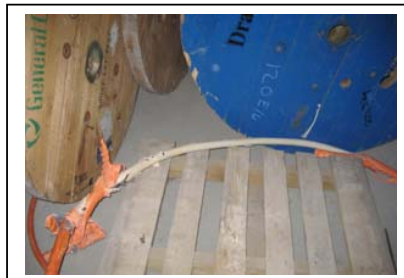
View of orange shield stripped away from 50mm fire rated cable.
