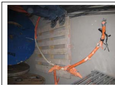
View of orange shield stripped away from 50mm fire rated cable.
