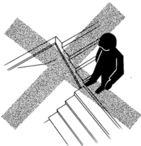
Figure 4 Unprotected stairways are a severe hazard.
