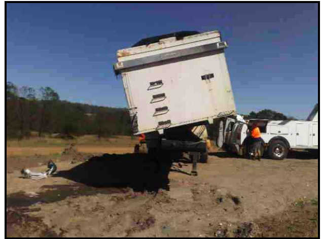
View Showing tipper trailer appears to have a twist
