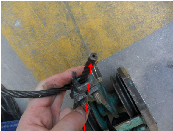
Termination end winch rope (hook end) showing rope having been cut
